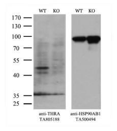
Equivalent amounts of cell lysates (10 ug per lane) of wild-type Hela cells (WT, Cat# LC810HELA) and THRA-Knockout Hela cells (KO, Cat# [LC810239]) were separated by SDS-PAGE and immunoblotted with anti-THRA monoclonal antibody TA805188. Then the blotted membrane was stripped and reprobed with anti-HSP90AB1 antibody ([TA500494]) as a loading control (1:500).
